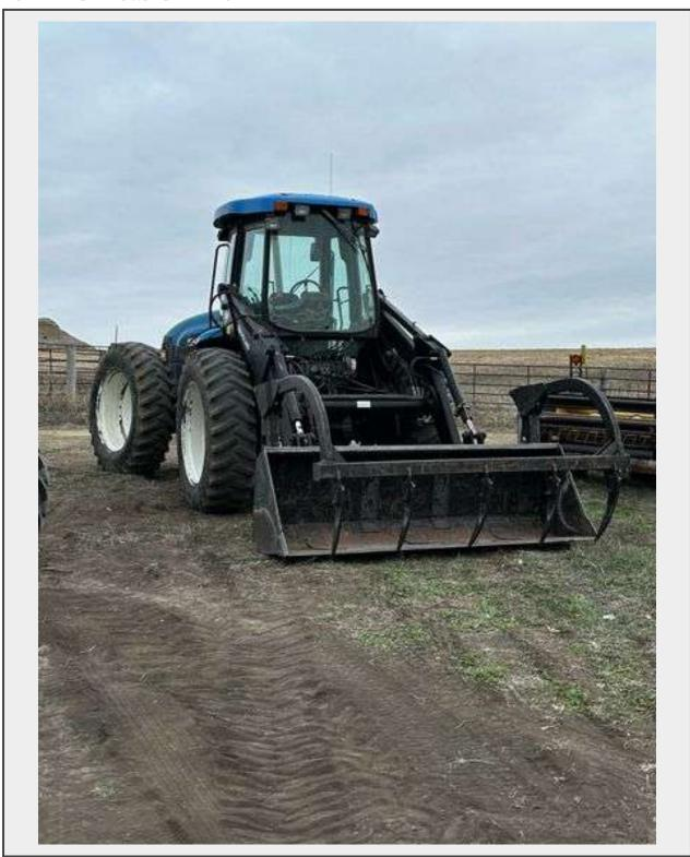
**Description**NEW HOLLAND TV140 w/loader, pto on both ends, wheel seals are leaking. 8010 hours
